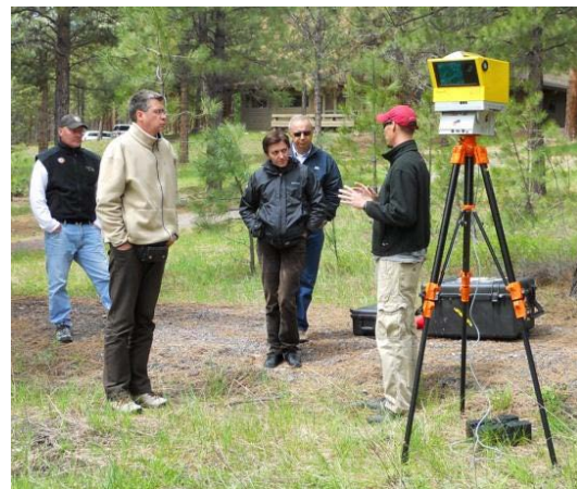
The Greek delegation gets a close look at terrestrial scanning LIDAR equipment used for three-dimensional mapping of fuel and vegetation, being demonstrated by Eric Rowell (right) of the National Center for Landscape Fire Analysis, University of Montana.
