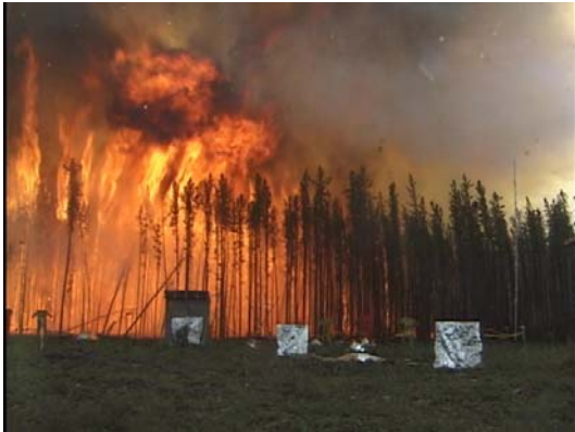
Figure 5--Plot 3 fire. Note that the fire is burning mostly on far right corner of the plot. The aluminum foil structures shown in the foreground are structure ignition sensor assemblies.
