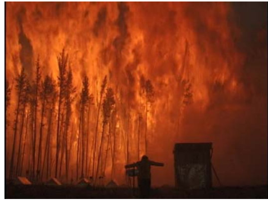
Figure 7--Plot 9 fire. Note that the flames are relatively large and uniform. The flame height was visually estimated to be 30 m.
