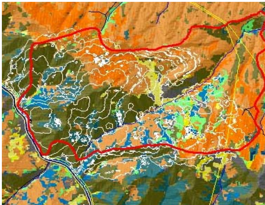
Figure 6—FARSITE simulation of Price Canyon Fire using gridded winds. Red line represents final fire perimeter, white lines represent predicted fire progression, note much closer match between actual and predicted perimeter (underprediction in top right is due to burnout operation and was not simulated in FARSITE).
