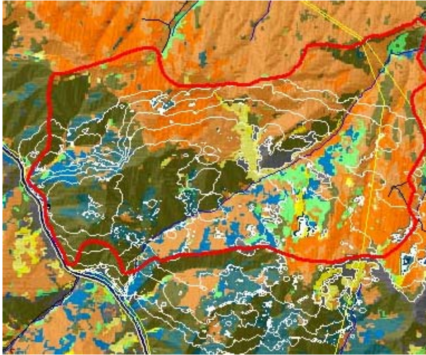
Figure 5—FARSITE simulation of Price Canyon Fire using uniform winds. Red line represents final fire perimeter, white lines represent predicted fire progression, note underprediction of fire spread in top left and overprediction along lower boundary of fire.
